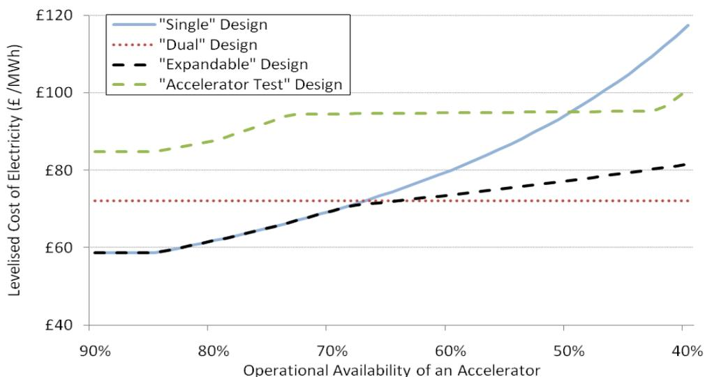
Figure 5: Levelised Cost of Electricity Production per MWh of electricity sold for two different flexible first-of-a-kind ADSRs compared to inflexible designs of one or two accelerator systems. Costs are in 2006 money.
