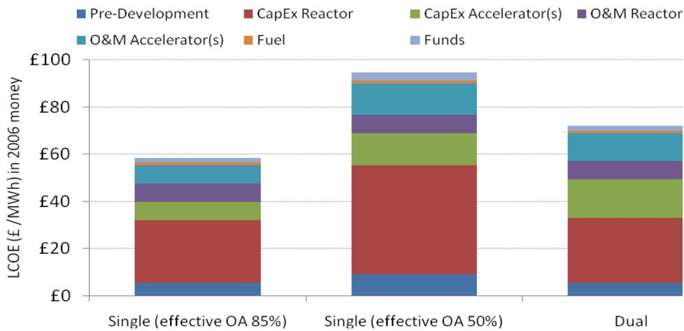
Figure 3: LCOE breakdown for the Single design at two different accelerator effective OA values and the Dual design, in the reliability regime where the Single design can be considered. In the figure “funds” refers to the money set aside for the combined geological disposal and decommissioning; and O&M stands for Operation and Maintenance.
