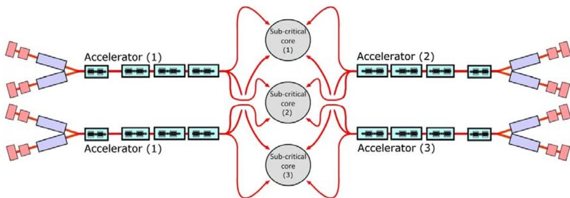
*Figure 7: Concept diagram for the suggested reactor park with an integrated network of accelerators and reactor cores. The numbers in brackets indicate in which of the three construction phases the reactor or accelerator is constructed. This diagram has been modified from reference (Pierini, 2007).*
