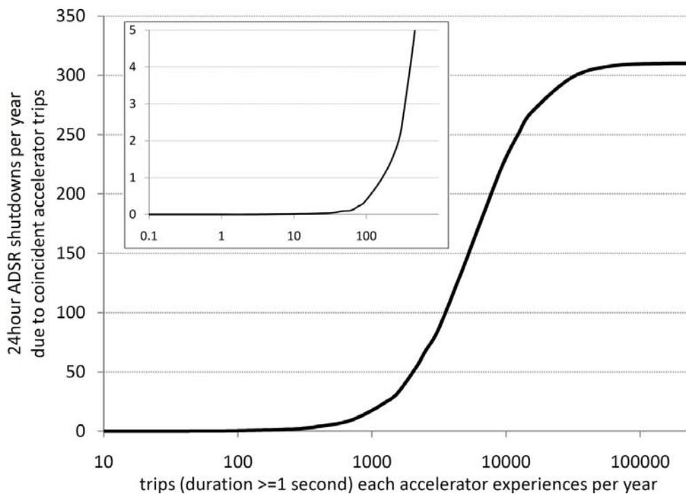
Figure 2: Annual number of coincident accelerator trips of duration  $\geq 1$  second for two accelerators for  $OA_{accel} = 85\%$ . Coinciding trips cause a 24 hour shutdown of the ADSR. Inset is the same data for a different range. A single contemporary seasoned accelerator at a research facility is expected to experience  $\sim 7500$  trips per year, while operating for only  $OA_{accel} \approx 70\%$ .
