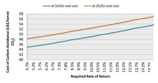
Figure 2. Estimated Cost of Carbon Avoidance (or required price of carbon) to finance CCS at a USCPC Power Plant in China under Varied Required Return Assumptions (Coal Price is \$4/GJ and 5\$/GJ, no carbon emissions cost and no financial leverage)
