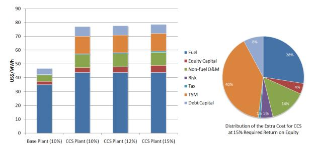
Figure 4. Structure of Required on-grid Tariffs for Financing a CCS Power Plant in China with 75% debt financing (with 6% fixed rate loan; 10%, 12% 15% required rate of return on equity and \$4/GJ coal cost assumptions, and no carbon market)
