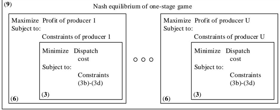
Figure 1: The derivation of one-stage game model under nodal pricing, mathematical formulations of each box is stated in bold fonts in paranthesis
