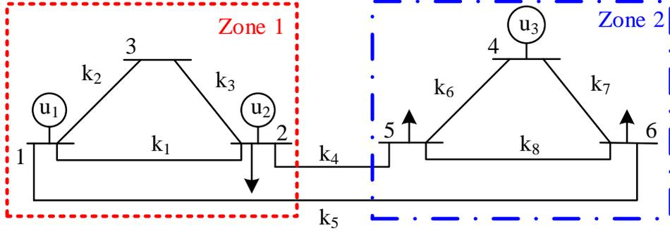
Figure 5: Single line diagram of 6-node example system
